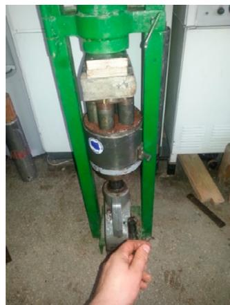
Figure 2. Preparation of specimens from the red clay–rubber (RC-R) mixture.
