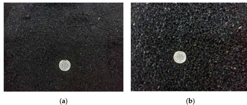
**Figure 1.** Rubber waste: (a) powder (P) 0–1 mm; (b) granulate (G) 1–5 mm.
