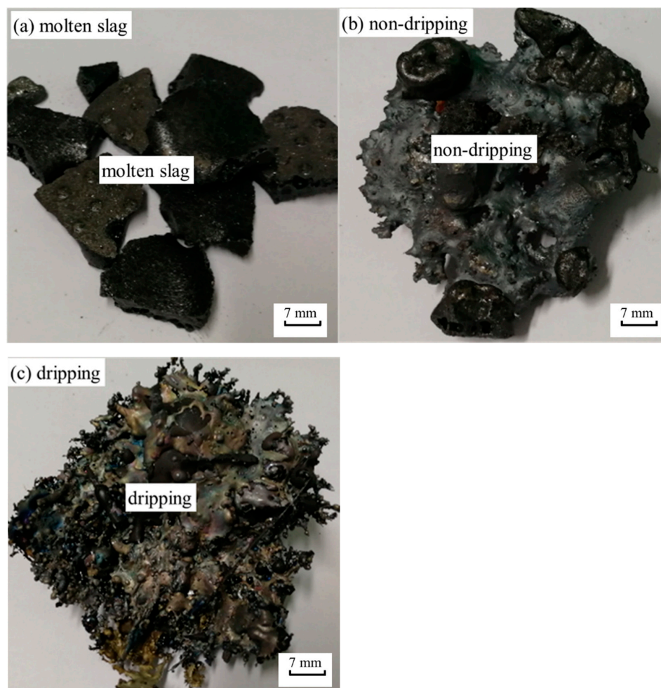
Figure 3. The macroscopic morphology of samples: (a) molten slag; (b) non-dripping; (c) dripping.
