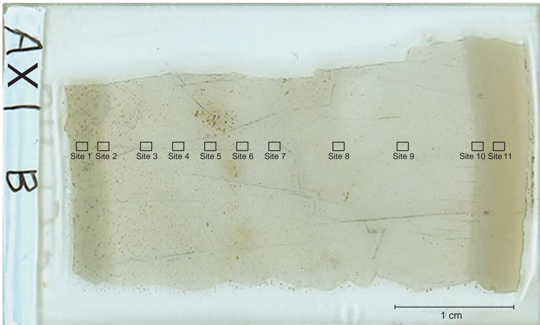
Figure S1.1: AX1B thin section showing respective sites taken for mineral chemical analyses (EDS) via Scanning Electron Microscope (SEM).
