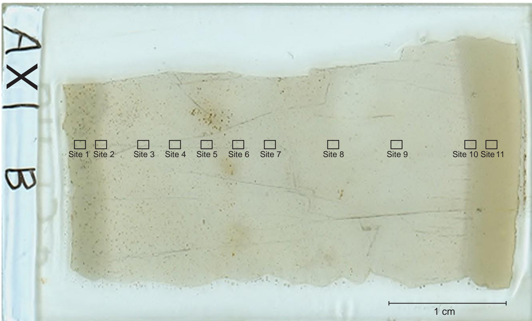
Figure S6.1: AX1B thin section showing respective sites taken for mineral chemical analyses (EDS) via Scanning Electron Microscope (SEM) (zooms in Appendix A1).
