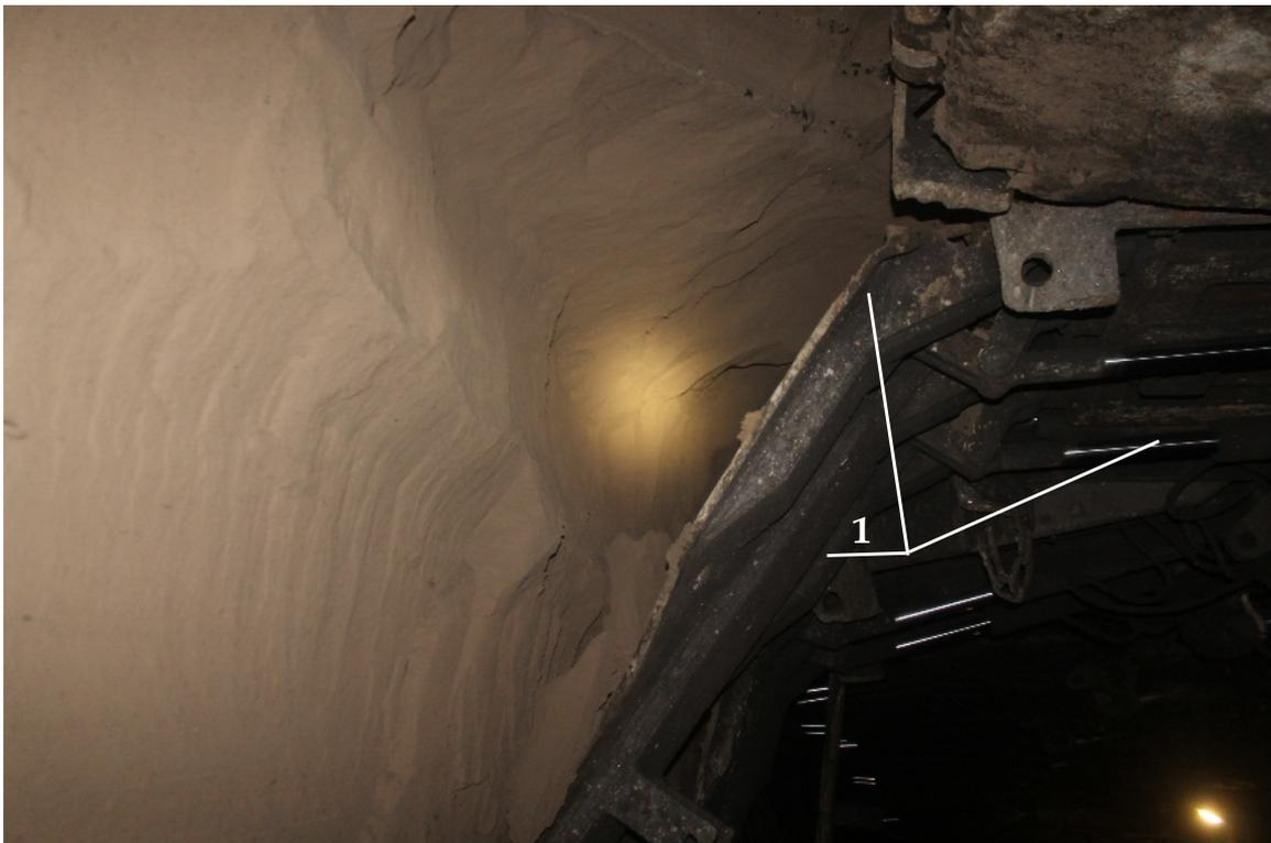
**Figure 4.** Exposed upper part of the incline filled with hydro-mixture based on fluidized ash; (1) upper elements of the powered roof support of the longwall complex.
