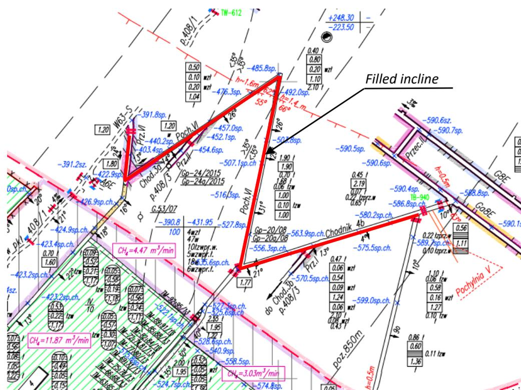
Figure 2. View of the incline filled with binding material made on the basis of fluidized ash.
