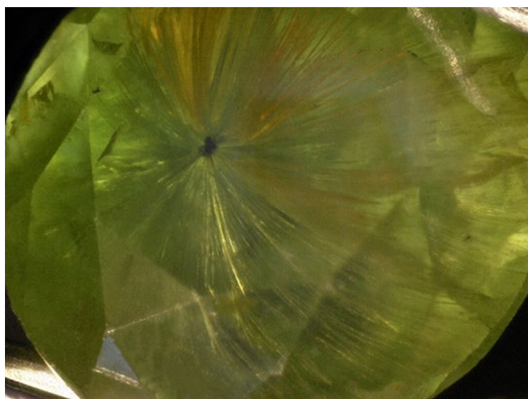
Figure 2. “Horsetail” inclusions in the demantoid from the Bobrovka river placer (Elizavetinskiy village, the Central Urals); image width 4 mm. Photo by E.S. Karaseva.
