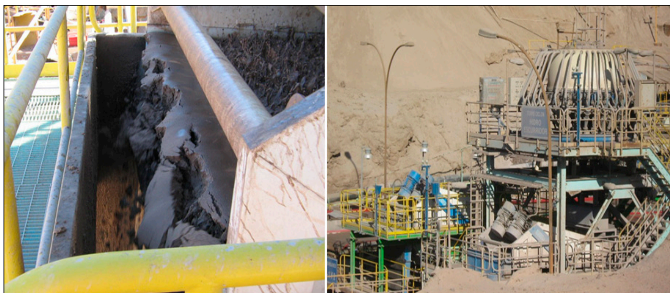
Figure 7. 2nd Industrial Trial Phase of Mantos Blancos Tailings Plant 8000 mtpd: Hydrocyclone Cluster + 02 Horizontal Vibratory Dewatering Screens [40,41].
