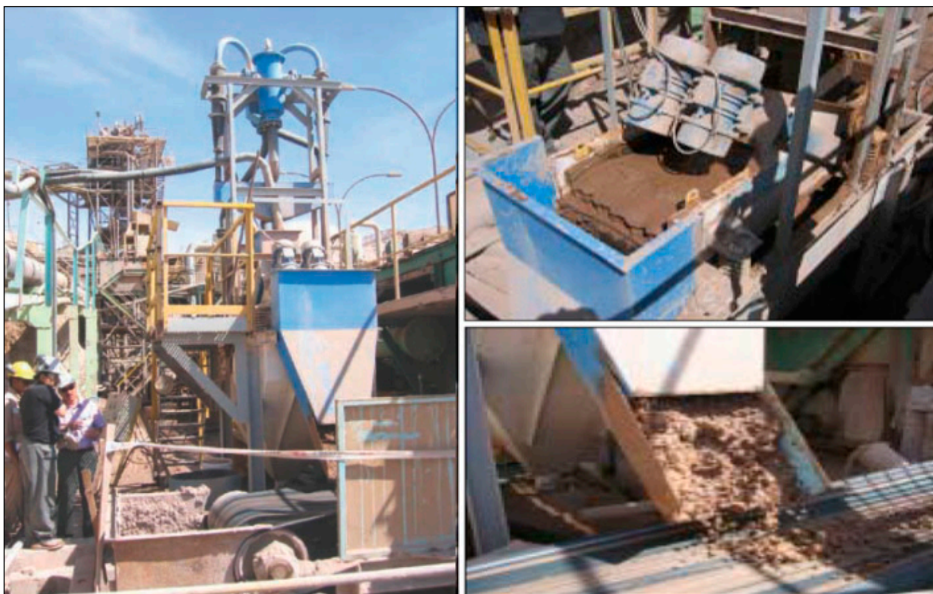
Figure 5. Dewatering Pilot Plant 600 mtpd: Hydrocyclone + Horizontal Vibratory Dewatering Screens Overview–Horizontal Vibratory Screens Operation–Cake Tailings Product [34].
