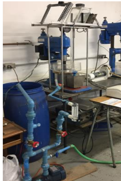
Figure 2. Gas dispersion testing rig. (a) Illustration, (b) photograph of the actual setup.
