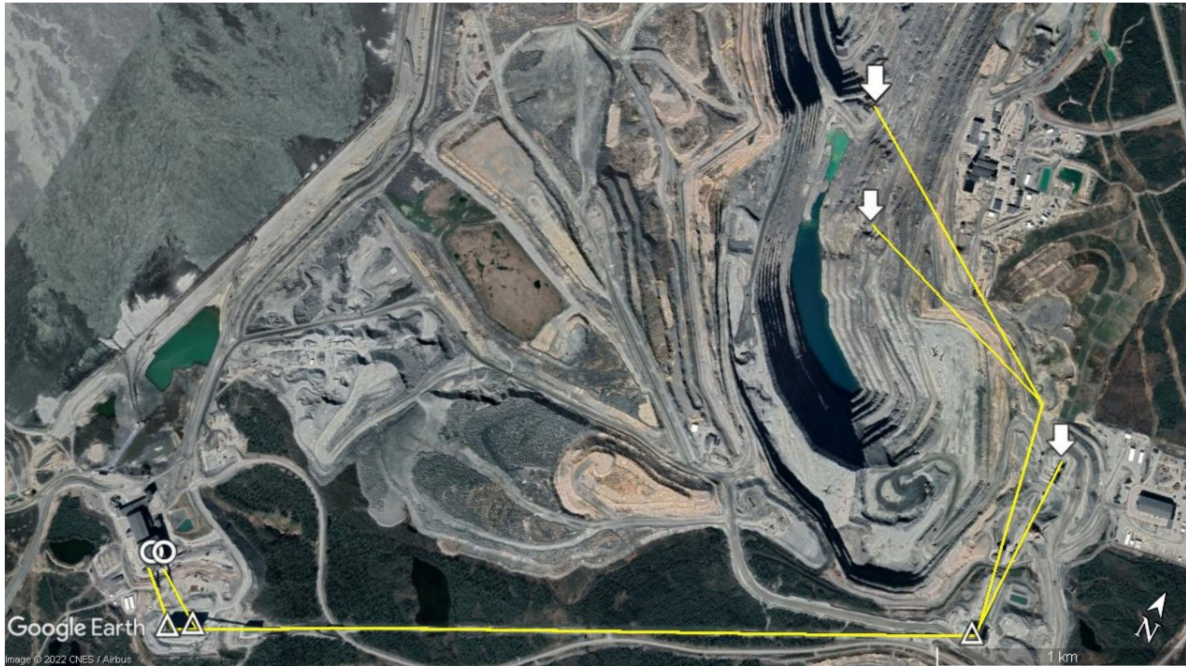
Figure 1. Overview of the southeast part of the mine, with the crushers, stockpiles, and the mills marked with white arrows, triangles, and circles, respectively. The yellow line shows the approximate trace of the conveyors. Created with Google Earth Pro.
