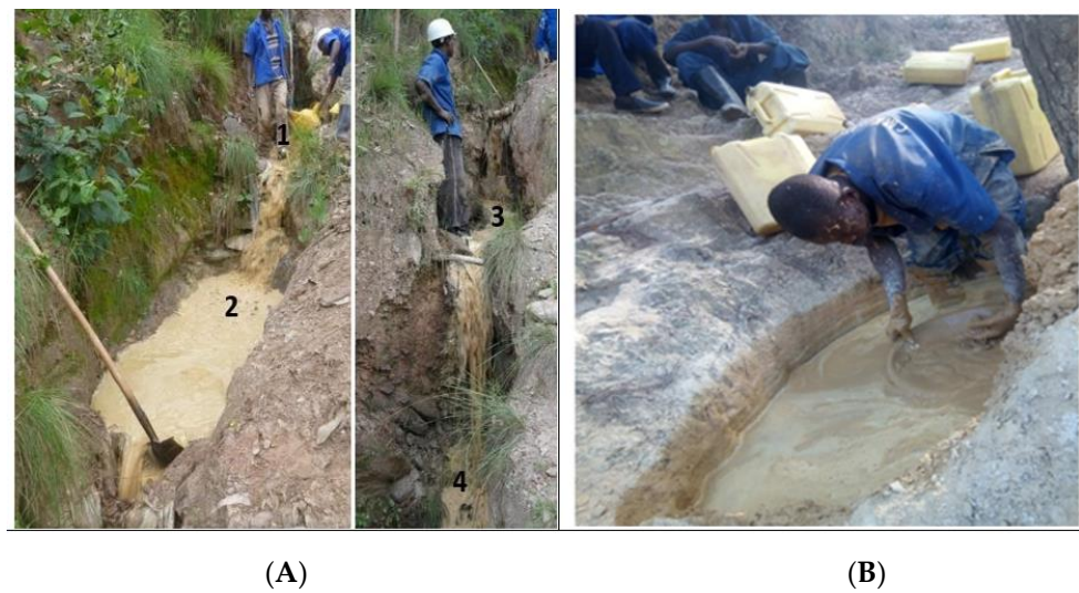
Figure 2. The general ground sluicing method (A) [1] and panning method (B) of Company X.
