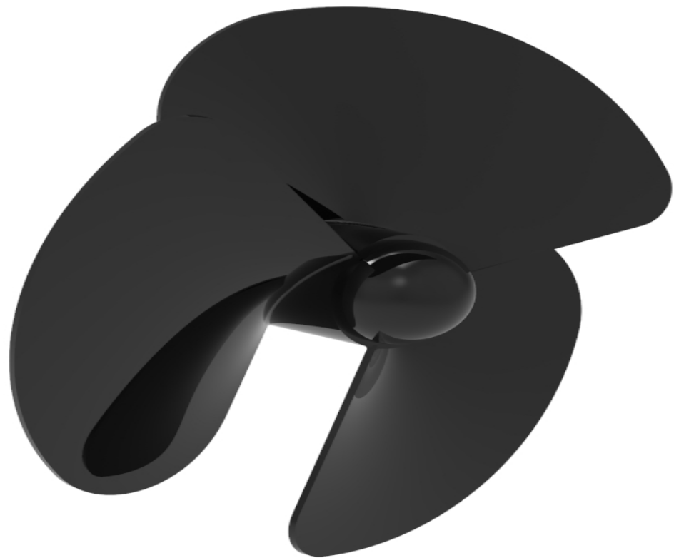
Figure 9. A typical representation of VTOL Propeller of Co-axial propulsive system.
