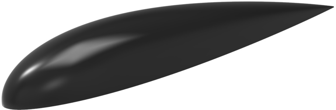
Figure 2. A typical isometric representation of fuselage.
