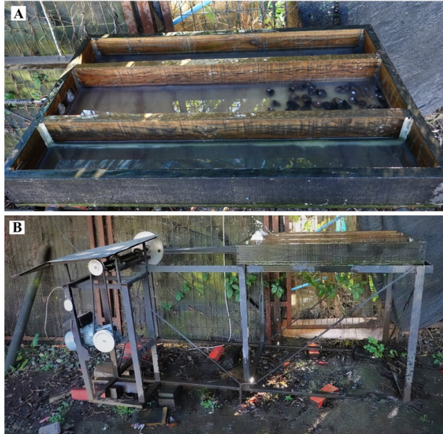
Figure S2: A: Upper part of the oscillatory box, divided into three equal parts to allow the clasts to move mainly in the direction of the major axis of the box; B: a view of the three-phase motor type ML 7114, and the series of pulleys to decrease the angular velocity and a pulley with an eccentric connector to transform the rotary movement into an oscillating one.
