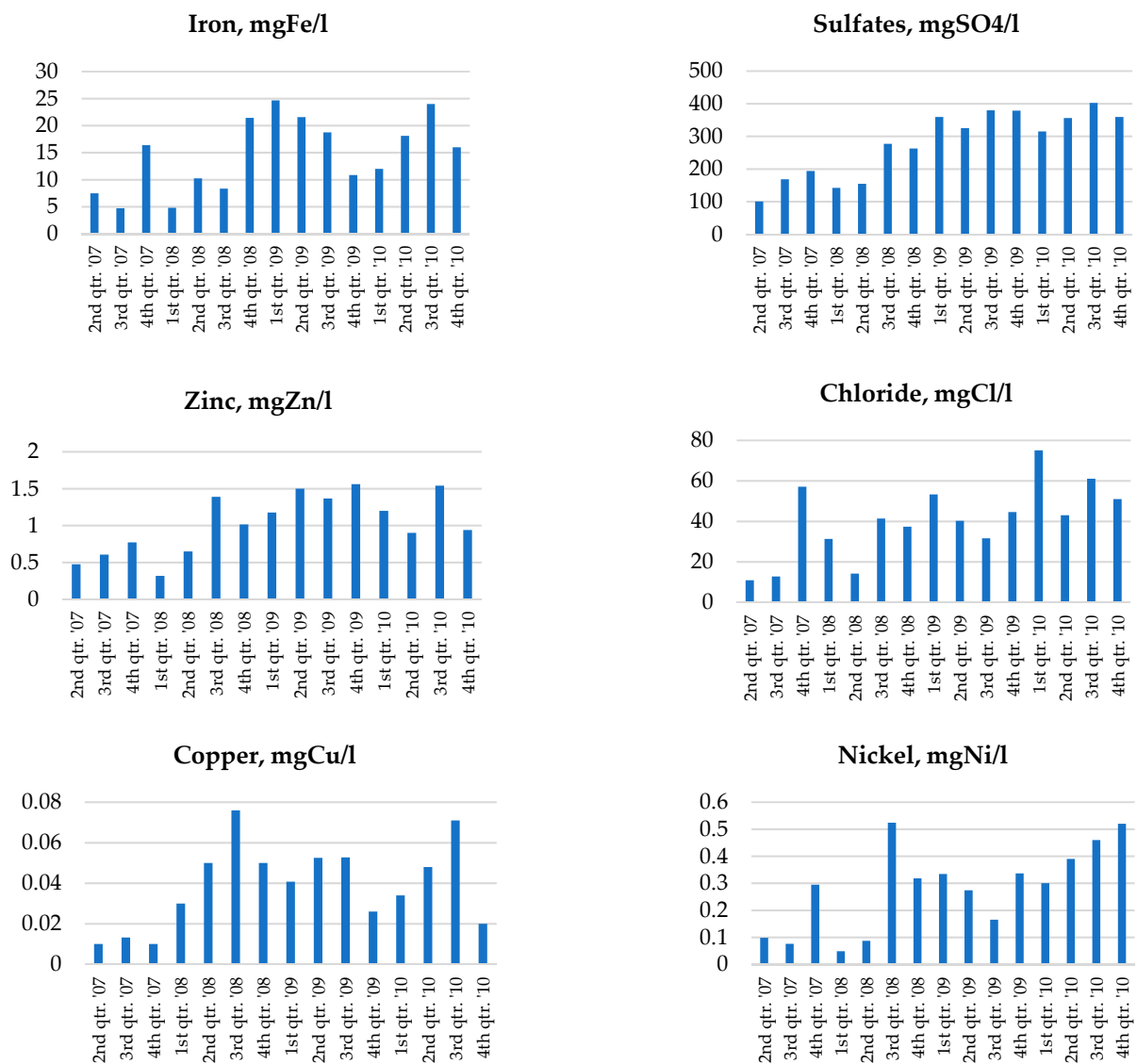
Figure 3. Average values of metallic elements in water collected from piezometers P 12, P 15, P 16, P 17 (April 2007 to December 2010).
