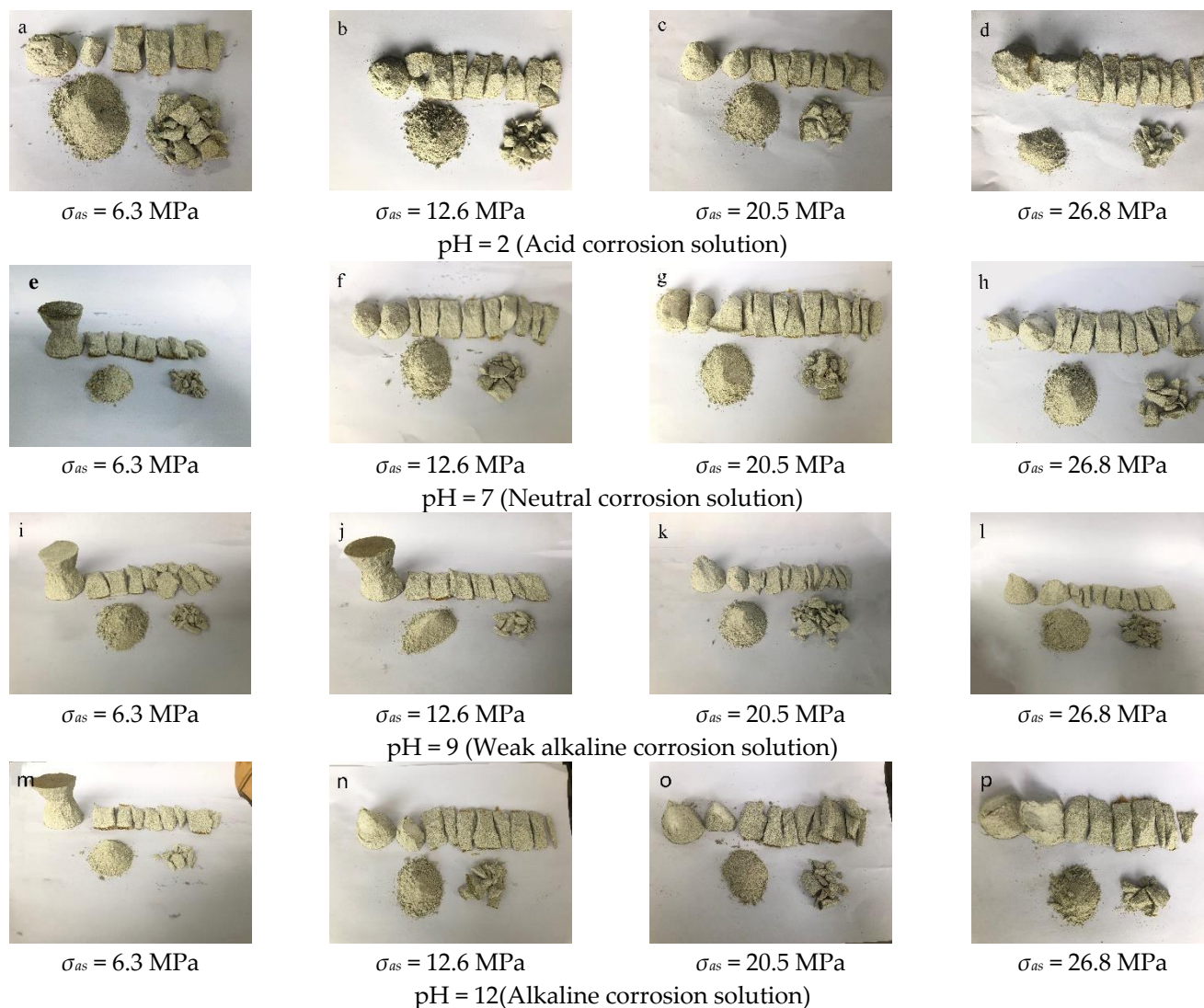
Figure 9. The destructed forms of white sandstone (a–p).
