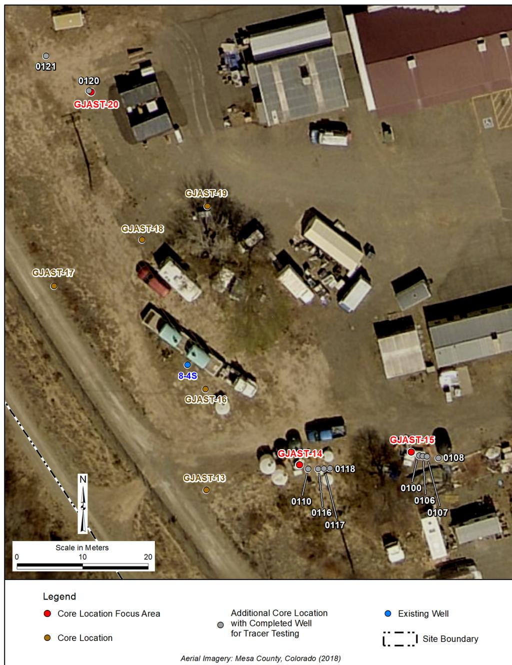
**Figure 3.** Zoomed-in image from Figure 1 around well 8-4S showing additional coring locations that were used for sediment compositing. Wells were completed in these coring locations for subsequent tracer testing.
