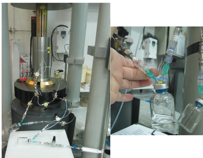
Figure 4. Squeezing technique for collecting the pore water from bentonite blocks.
