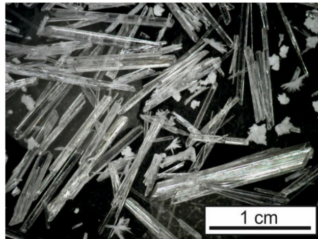
Figure 12. Clear untwinned crystals of gypsum, \text{CaSO}_4 \cdot 2\text{H}_2\text{O} , grown in silica gel with \text{AlCl}_3 additive.
