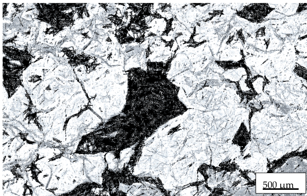
Figure 16. Typical microstructure of a microwaved sample of bauxite ore (2) showing the cracks ( \times 450 ).
