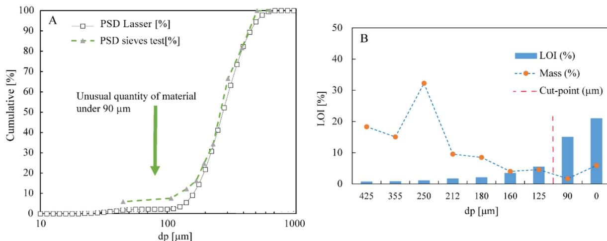
**Figure 5.** (A) Particle size distribution of the initial material resulted from the laser analysis and sieve analysis, where the cumulative mass is plotted against particle diameter, (B) LOI (%) content for each particle size range in abscissa.
