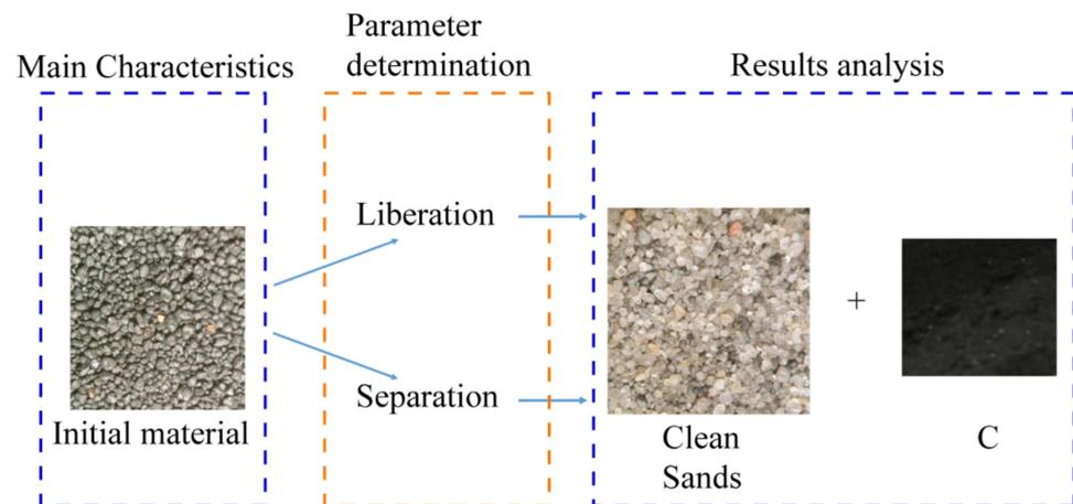
**Figure 1.** Work strategy scheme to evaluate liberation performance. In an initial stage we have raw material. After liberation and separation, the obtained material is a clean sand plus the removed volatile matter, which is mainly carbon.
