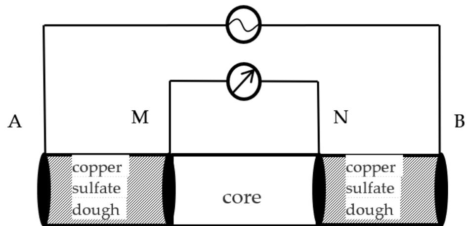
**Figure 2.** Schematic diagram of the complex resistivity measurement of the rock samples.
