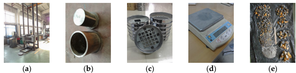
Figure 2. The experimental equipment and result: (a) hydraulic press; (b) indenter and experimental cylinder; (c) standard stone sieves; (d) electronic scale; (e) crushed particles with different sizes.
