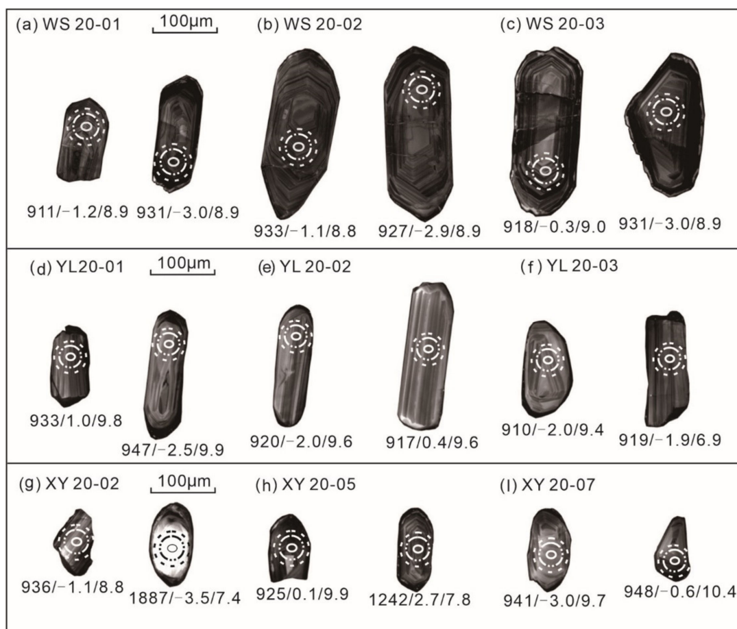
Figure 6. Representative zircon CL images with ages/ \epsilon_{\text{Hf}}(t) / \delta^{18}\text{O} values for the granitic mylonites from Wushan (a–c) and granitic gneisses from Yuanlong (d–f) and Xinyang (g–i) in the western margin of the NQT. The smaller circles 10 \mu\text{m} in diameter, the medium circles 30 \mu\text{m} in diameter, and the dashed circles 40 \mu\text{m} in diameter represent analytical sites for the O, U–Pb, and Lu–Hf isotope determinations, respectively.
