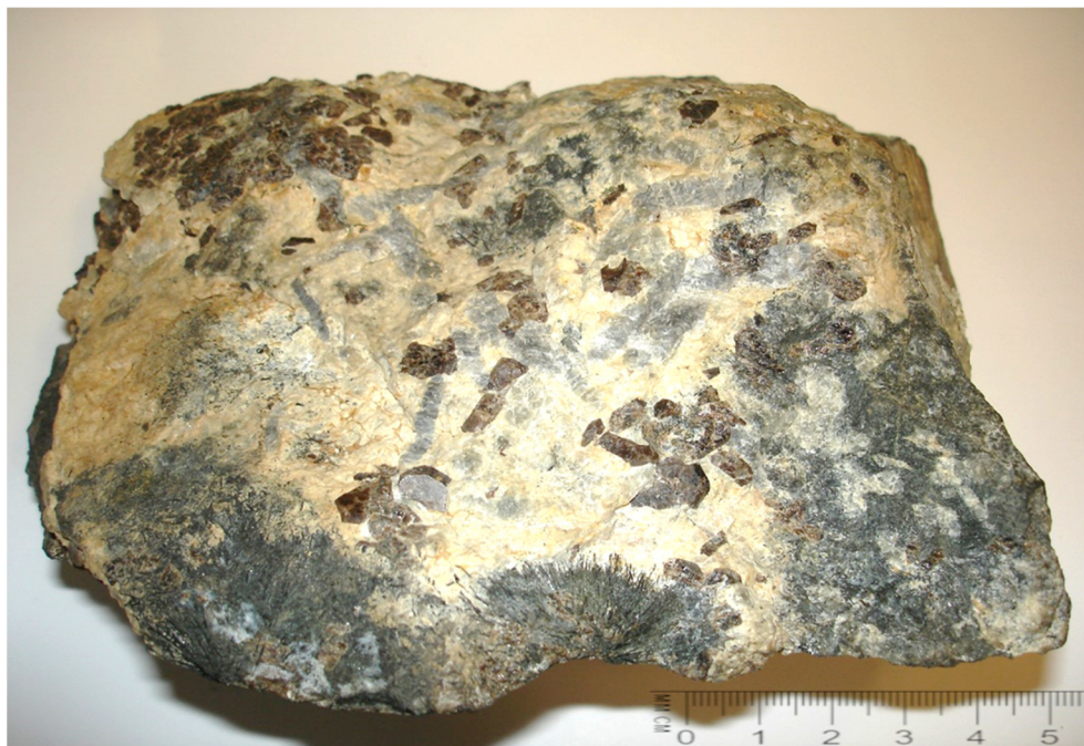
Figure 3. The sample of Odikhincha peralkaline pegmatite (17 × 14 cm). Coarse-grained part: EGM—reddish-brown, orthoclase—gray, nepheline and hydroxycancrinite mass—pale yellow, aegirine—black, fine-grained aggregates—dark-gray.
