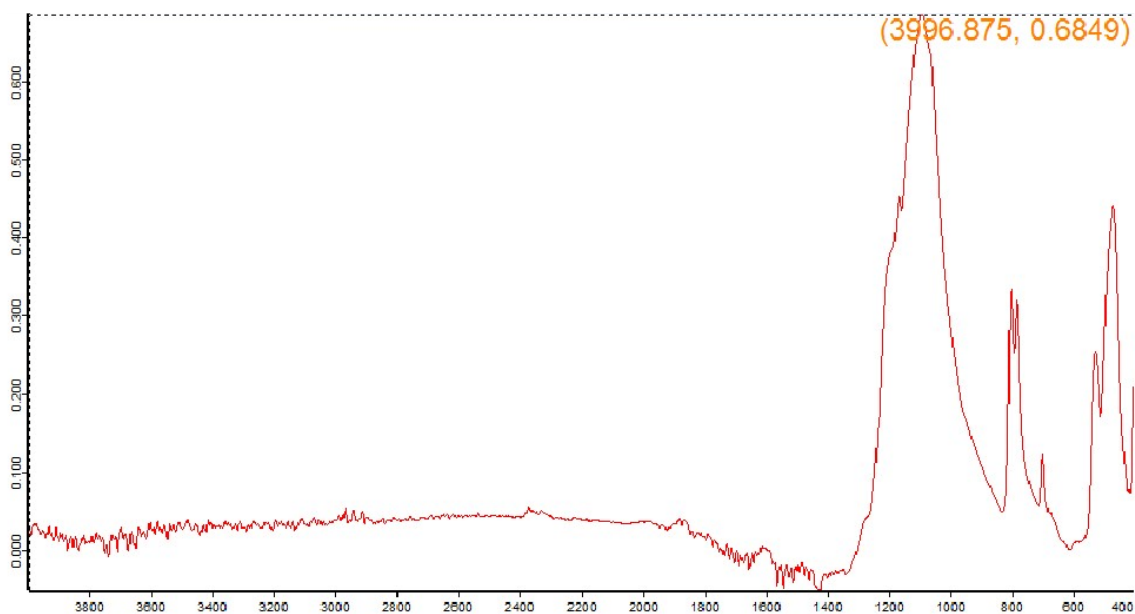
Figure S4. Example infrared spectrum on a pure silica dust sample using the portable Bruker Alpha II FTIR instrument and OPUS software (Version 8.2.28, 32 bit).
