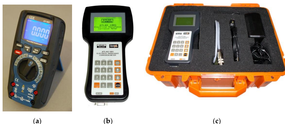
Figure 11. Meters fitted in the protection system: (a) multimeter for potential measurements, (b,c) ATLAS 1001 COR resistive corrosion meter with accessories.
