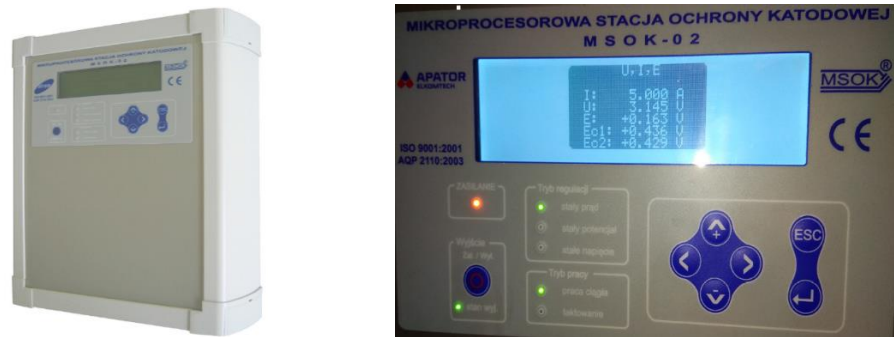
Figure 4. View of the MSOK-02 microprocessor cathodic protection station and its control panel.
