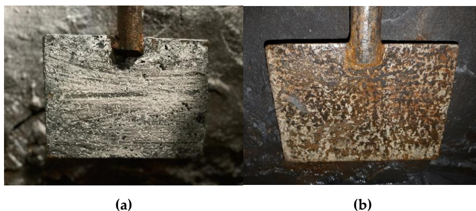
Figure 15. View of the reference plate installed inside the classifier tank: (a) plate with cathodic protection, (b) plate without cathodic protection.
