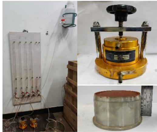
**Figure 2.** Permeability test apparatus and test sample.
