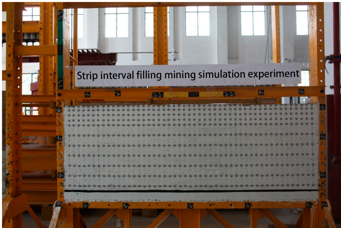
Figure 20. Model measurement point layout.
