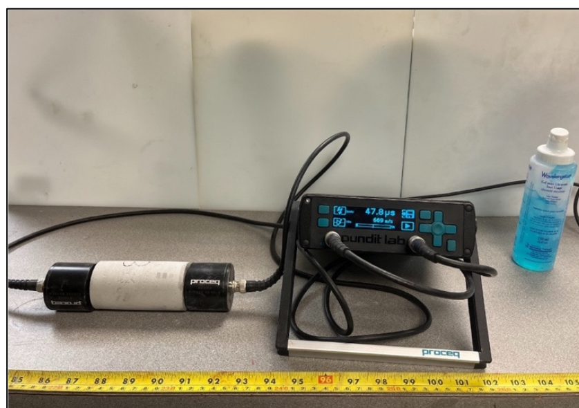
Figure 6. Experimental setup for ultrasonic pulse velocity measurement.
