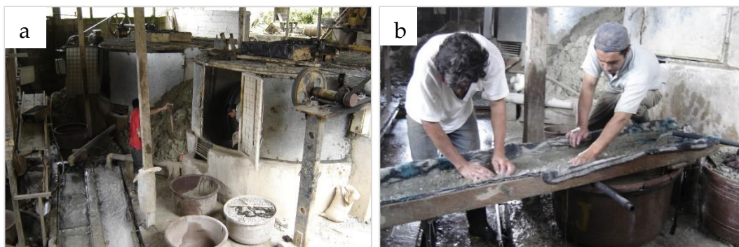
Figure 3. Settlement of the grinding–amalgamation cycle: (a) mineral concentration (mill washing), (b) traditional amalgam and mercury recovery from tailings.
