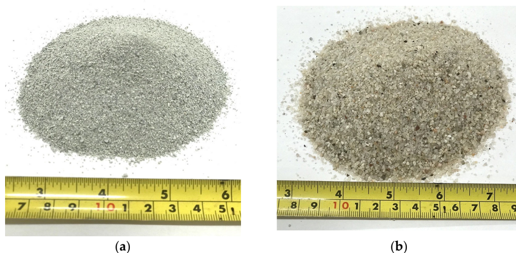
Figure 2. Materials used in this study: (a) bentonite; (b) sand.
