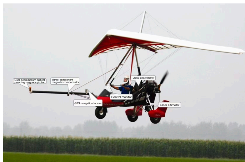
Figure 1. The dynamic delta wing aeromagnetic survey system in a low-altitude range.
