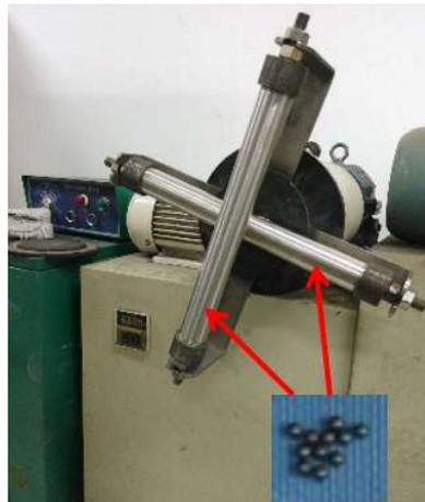
**Figure 2.** Micro-strength tests equipment.
