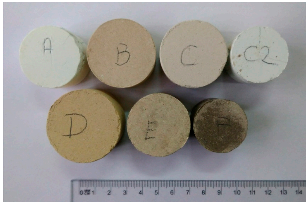
Figure 6. Appearance of the materials obtained after synthesis at 1350 °C for 8 h.
