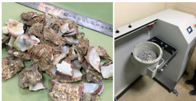
Figure 1. Photo of the waste seashells and grinding mill used.
