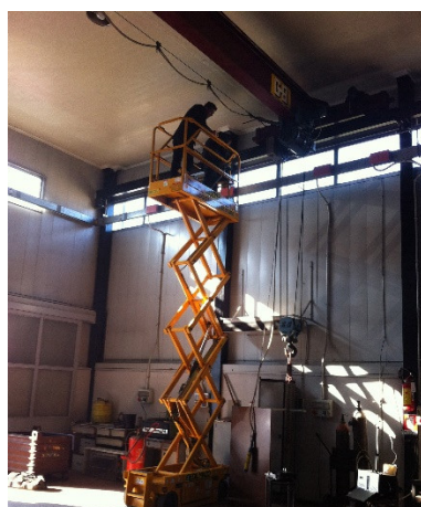
Figure 3. Overhead crane present in building A. The figure shows two operators on lifting platform collecting samples of dust settled on the overhead crane.
