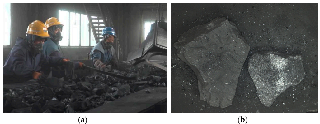
Figure 2. The picture of the manual sorting scene and the sorted coal gangue. (a) Manual sorting; (b) sorted coal gangue.
