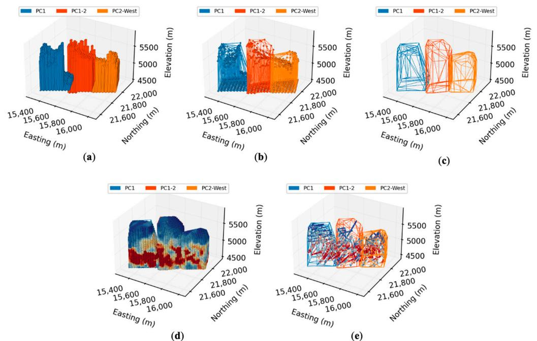
Figure 3. Creating convex hulls for panel caves and locating data points: (a) Cave drawpoints with BHOD; (b) Constructing convex hulls for panel caves; (c) Simplifying shapes of convex hulls before data selection; (d) Locating blocks within convex hulls; (e) Locating drill core composites within convex hulls.
