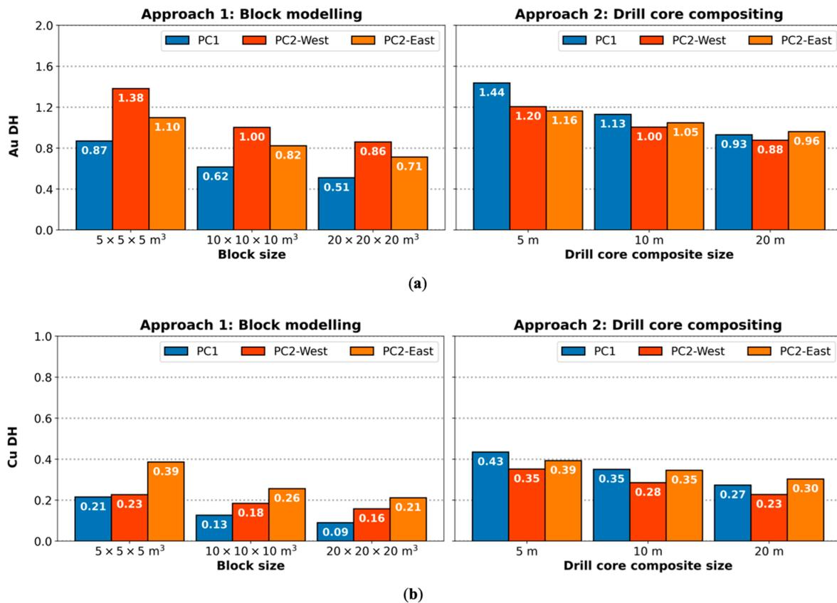
Figure 4. In situ gold and copper grade heterogeneities of panel caves estimated by block modelling and drill hole grade data sets: (a) Gold heterogeneity; (b) Copper heterogeneity.
