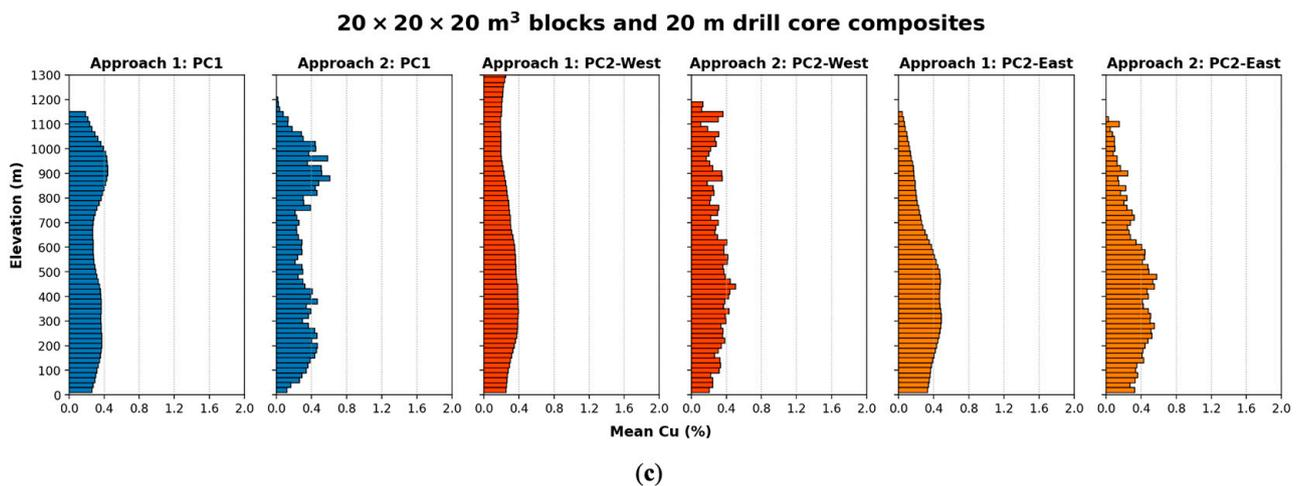
**Figure 6.** Change in copper grades of caves with elevation: (a) 5 × 5 × 5 m<sup>3</sup> blocks and 5 m drill core composites; (b) 10 × 10 × 10 m<sup>3</sup> blocks and 10 m drill core composites; (c) 20 × 20 × 20 m<sup>3</sup> blocks and 20 m drill core composites.
