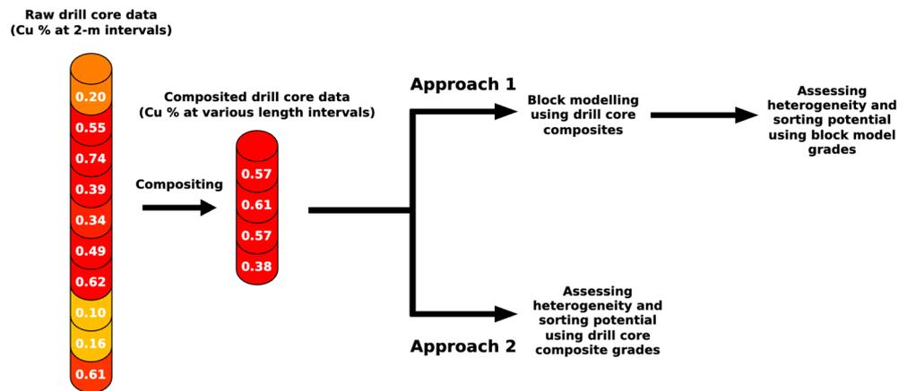
Figure 2. A schematic of block modelling and drill core compositing approaches.
