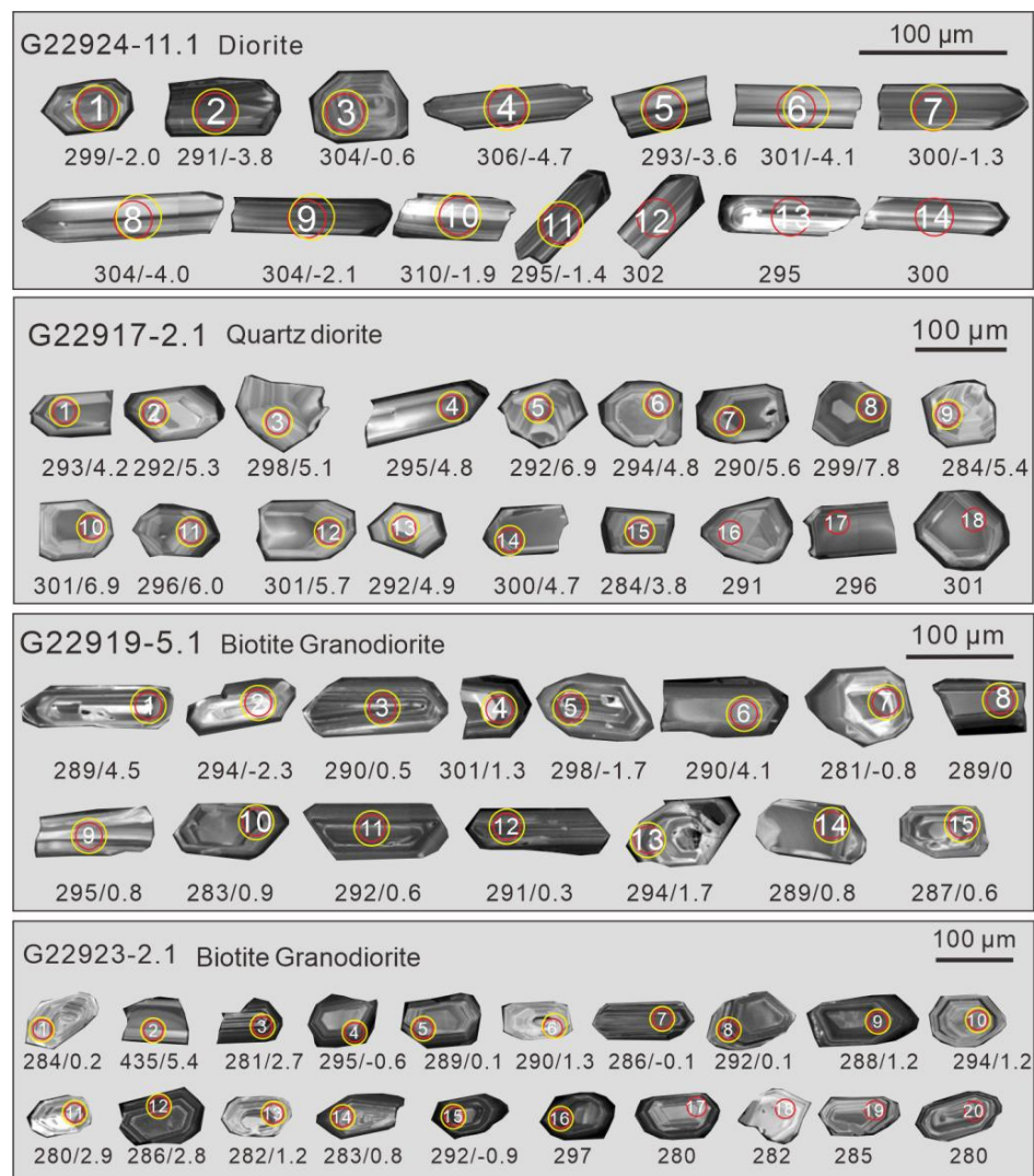
Figure 4. Cathodoluminescence (CL) images of the analyzed zircons. The red and yellow circles on zircons show the positions for U-Pb dating and Lu-Hf isotope analysis, respectively. The numbers below zircons represent ^{206}\text{Pb}/^{238}\text{U} ages and \epsilon_{\text{Hf}}(t) values, respectively.
