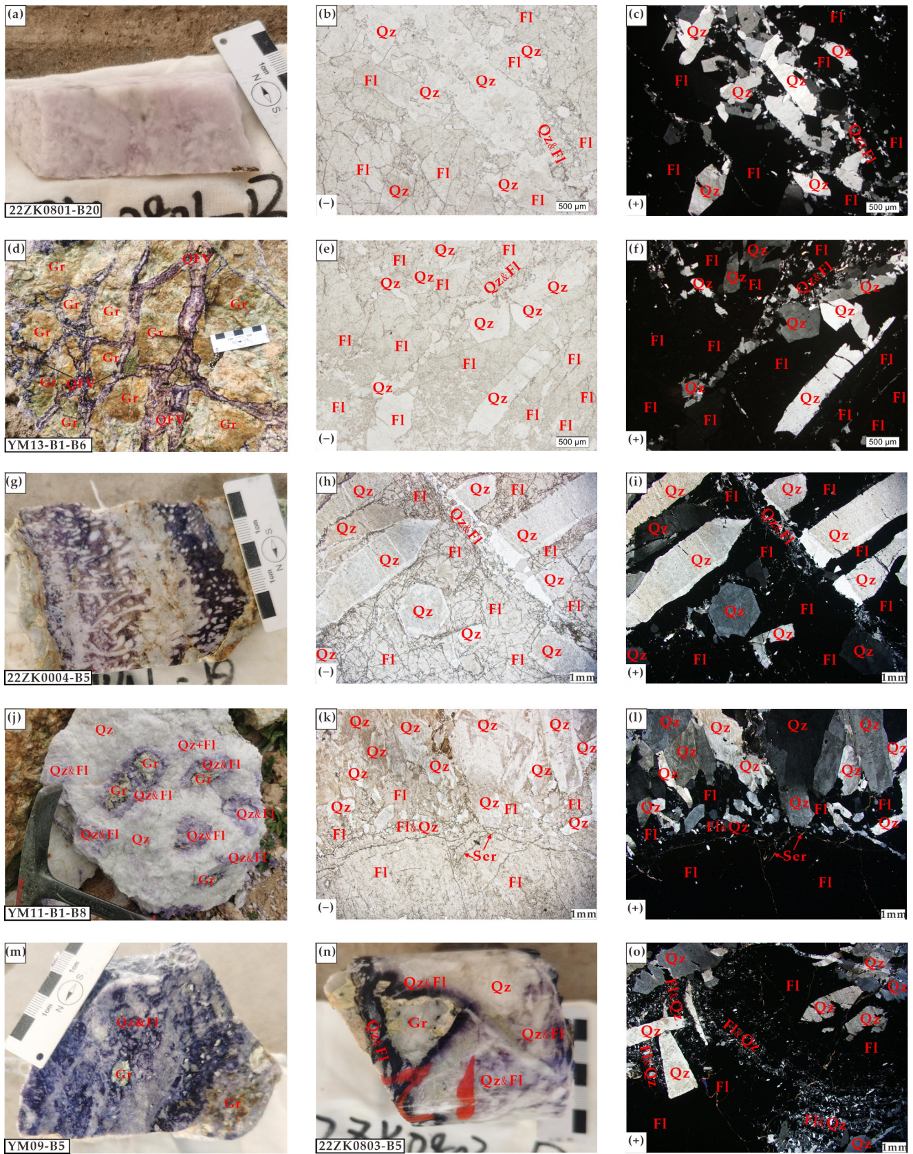
Figure 7. Photographs and photomicrographs showing the morphology and textural features of the fluorite ores in the Yama fluorite deposit. (a) Photograph and (b,c) photomicrograph of sample 22ZK0801-B20 of Type 1 ore; (d) photograph and (e,f) photomicrograph of sample YM13-B1-B6 of
