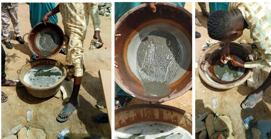
Figure 6. Manual amalgamation and filtration with a fabric to remove excess mercury.
