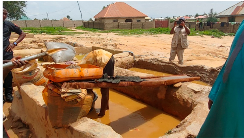
Figure 5. Gold concentration in sluice boxes at Uke mine site.
