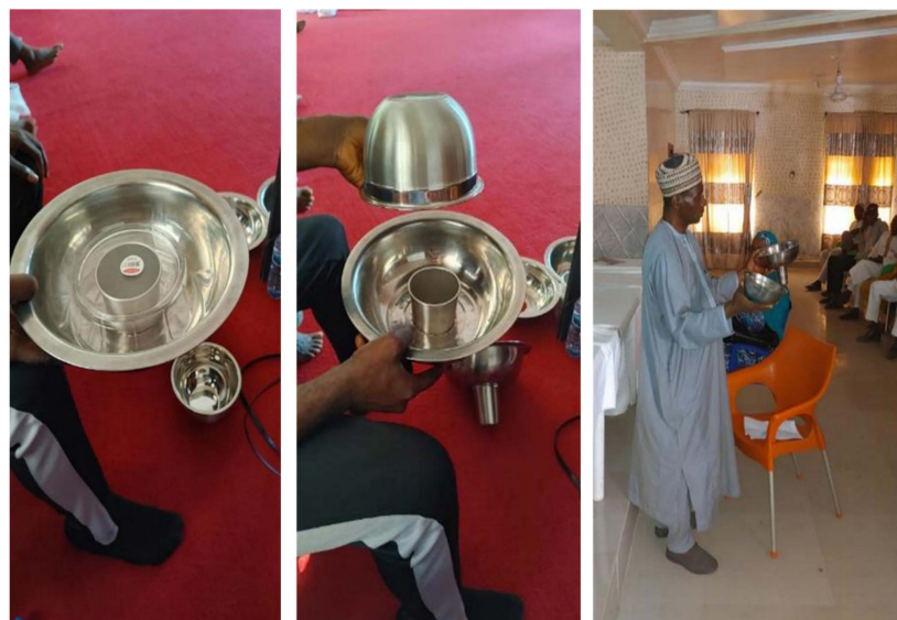
Figure 14. Salad bowl retorts made in Nigeria with glass and with stainless steel cover.
