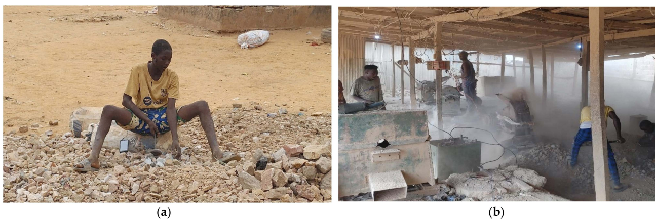
Figure 4. (a) Boy crushing ore and (b) dry hammer mills dry-grinding it below 1 mm.
