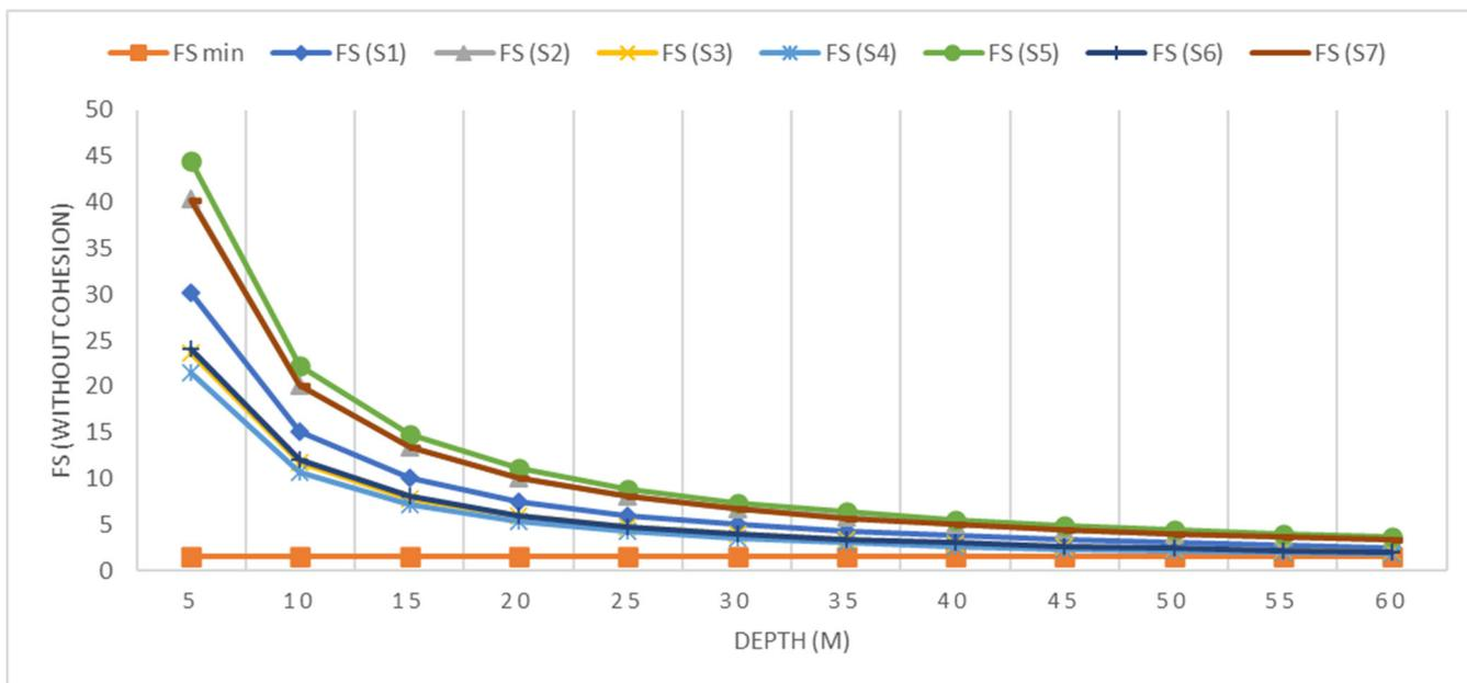
Figure 6. Variation of the safety coefficient according to the depth.
