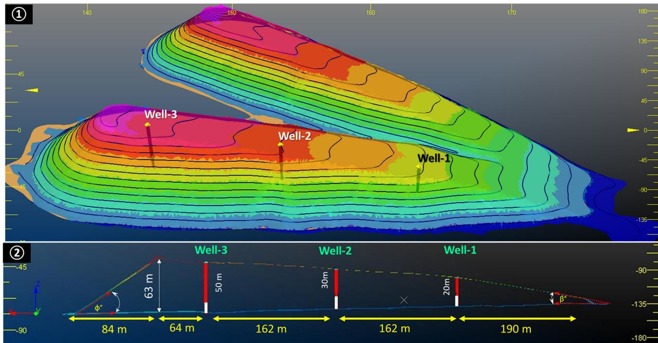
**Figure 3.** Arrangement of stockpiles and location of sampling wells; Legend: ① Perspective view (3D view) of the left arm of the screening PMWR stockpile; with the location of the three mining wells. It is noted that the well implantation mesh is around 162 m. ② Projection of the three wells on a longitudinal section representing the planned sampling depths by mining wells respectively (Well-1, 20 m, Well-2, 30 m, and Well-3, 50 m).
