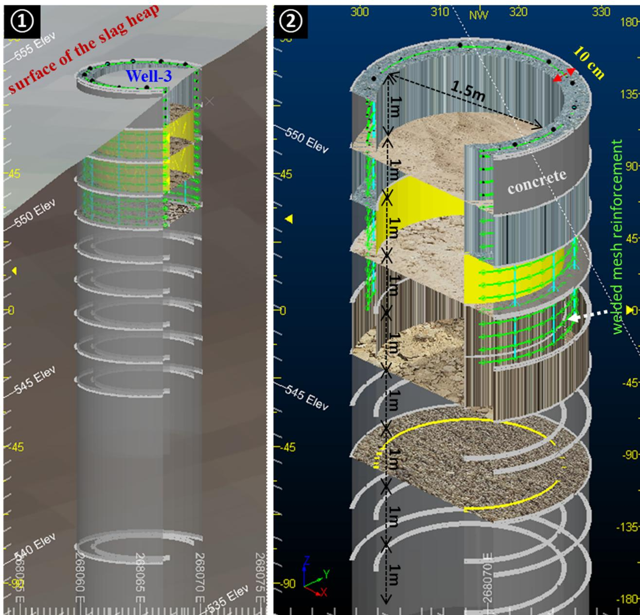
**Figure 11.** Representation of the design for mining wells: ① Localization of well-3 on the left arm of the screening PMWRS. ② Perspective view with a cross section (3D) of well-3 indicating the depth and walls supported by reinforced concrete, the diameter (1.5 m), and the thickness of the well support with concrete walls reinforced with welded mesh reinforcement.
