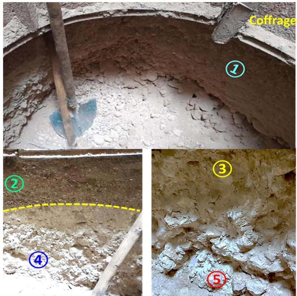
**Figure 13.** Lithological survey of the walls of well-1; Legend: ① Fine phosphate, ② Sandy, calcified and calcareous phosphate, ③ Calcified indurated phosphate, ④ Altered and calcified phosphate, ⑤ Fragments of indurated phosphate that have become friable, generating a sandy phosphate.
