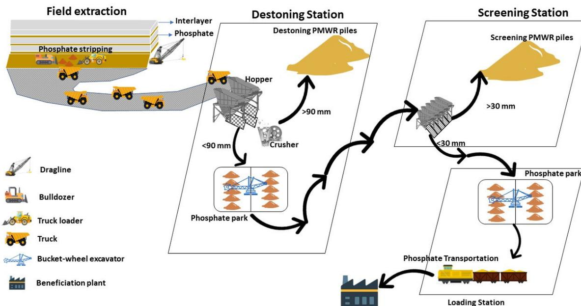
Figure 2. Phosphate extraction and Mining processing protocol in Benguerir prospect.
