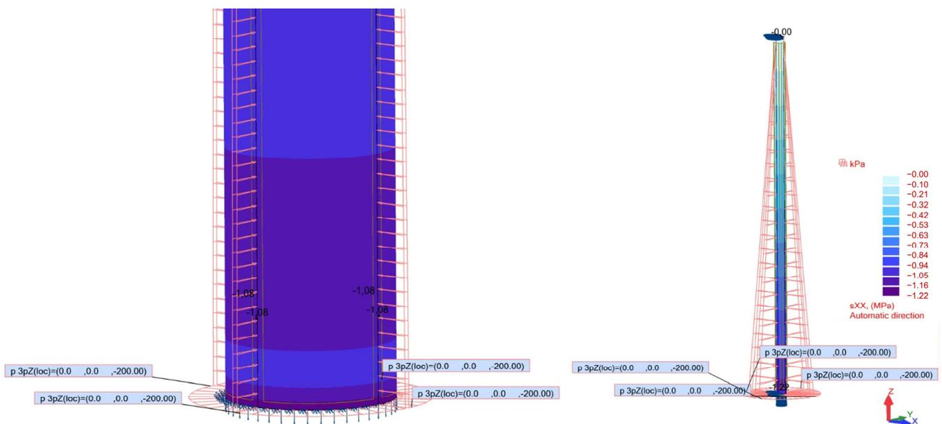
**Figure 5.** Results of the numerical modeling of the stress applied on the well.
