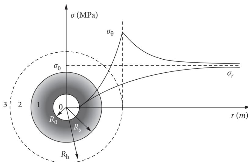
**Figure 4.** Stress distribution diagram of elastic-plastic zones of a well [27]; Legend: R<sub>0</sub>: Radius of the well; R<sub>s</sub>: Radius of plastic softening zone; R<sub>h</sub>: Radius of the hardening zone, 1: Plastic softening zone; 2: Plastic hardening zone; 3: The elastic zone.
