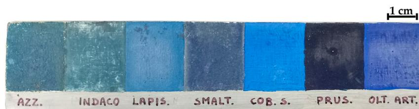
**Figure 2.** Mock-up panel painting of blue pigments. The pigment is indicated under each square. Azz.: azurite; INDACO: indigo; LAPIS.: Lapis lazuli; Smalt; COB. S.: cobalt blue; PRUS.: Prussian blue; OLT. ART.: ultramarine.
