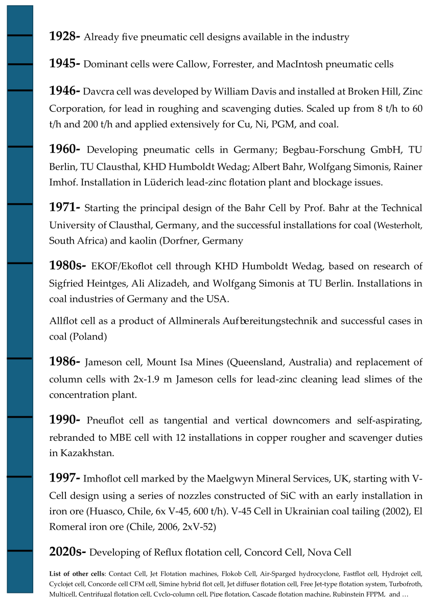
Figure 1. A historical overview of the development of pneumatic flotation cells [5,6].
