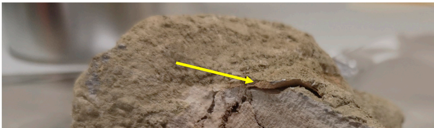
Figure 3. Laboratory-produced quicklime sample after calcination. Surface layer partially covering the surface is marked with yellow arrow.
