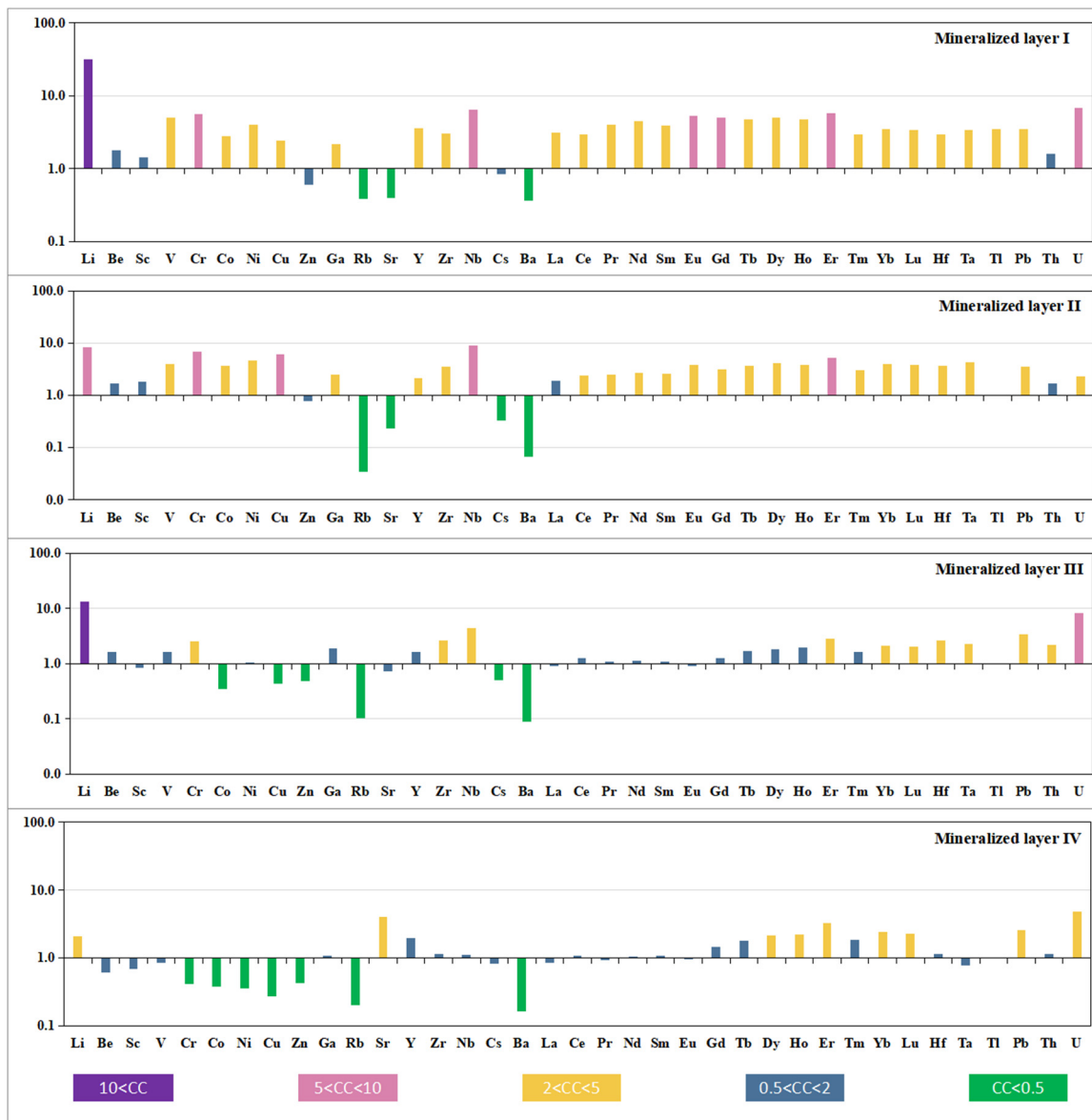
Figure 6. Concentration coefficients of trace elements of mineralized layers I, II, III, and IV in coal-bearing series from Wanfu mine, Xian’an coalfield, Guangxi Province.
