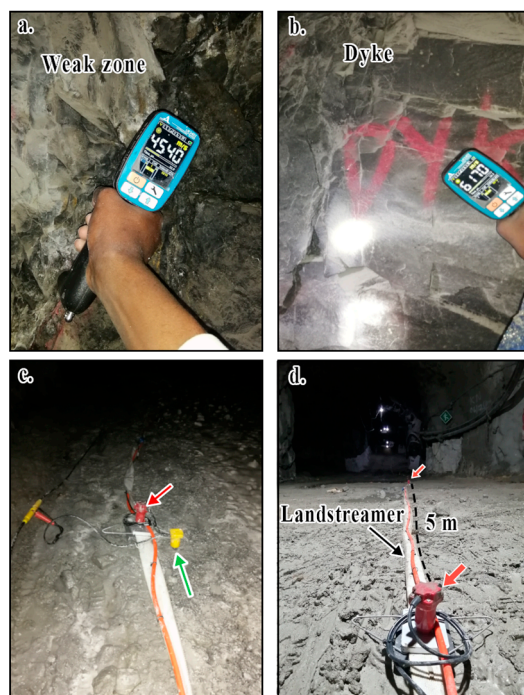
Figure 4. Measurements of the seismic velocities underground using an ultrasonic pulse meter over a (a) weak zone and (b) dyke. (c,d) Shows the setup inside the tunnel of the seismic survey using the seismic landstreamer (red arrows) and planted geophone (green arrows).
