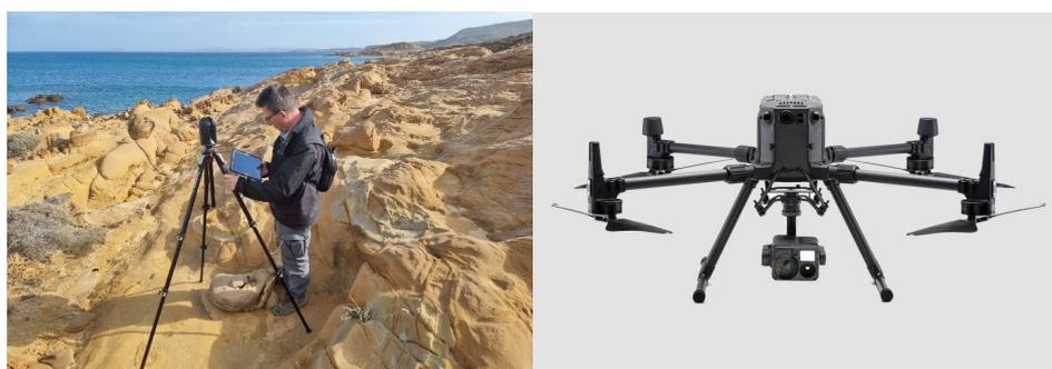
**Figure 2.** (a) Laser scanning survey using a Leica BLK360; (b) an indicative photo of the DJI Matrice 300 with a Zenmuse ZH20 camera on board.
