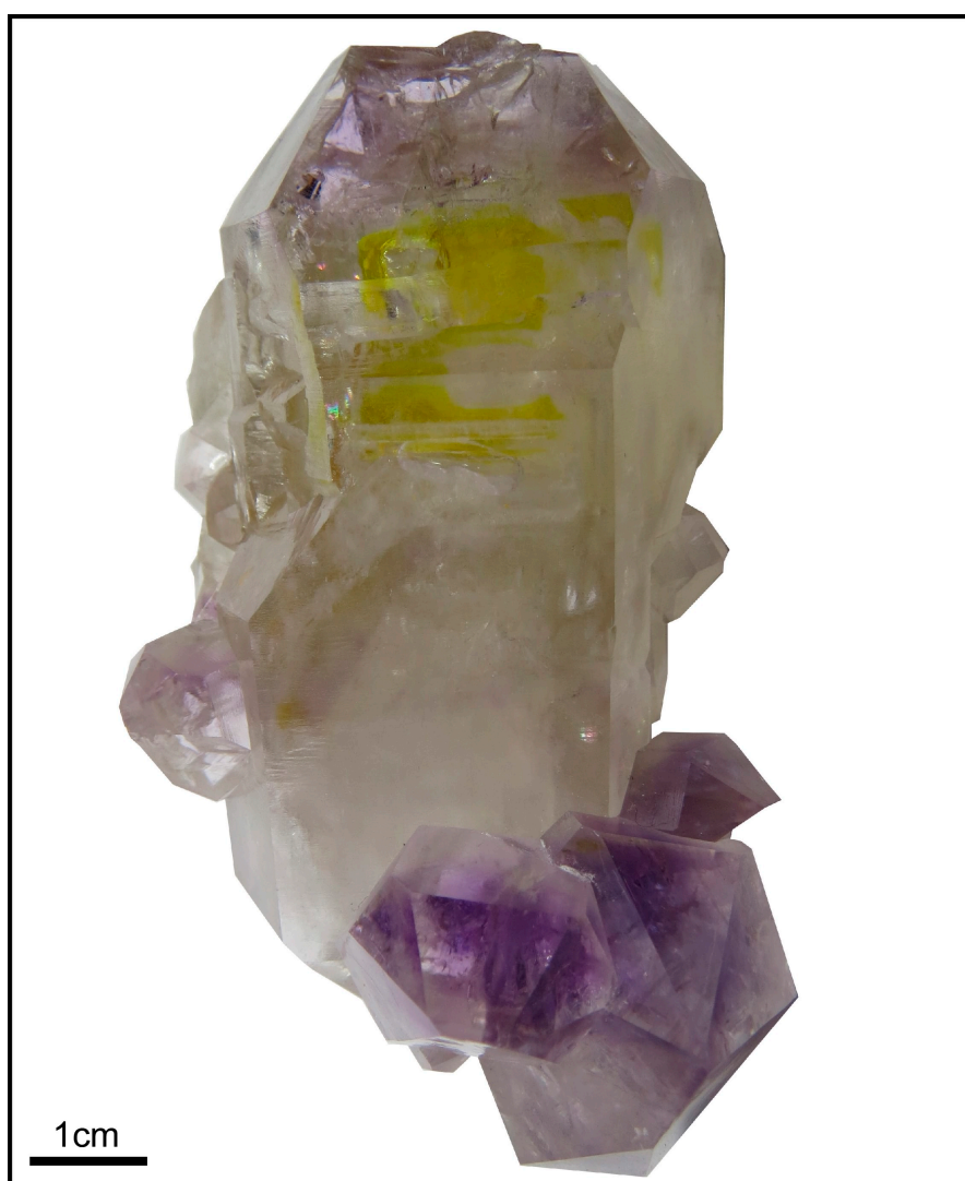
Figure 2. Photographs of a quartz-amethyst crystals with centimetric scale amber coloured oil inclusions (Type 3). The amber coloured phase in the inclusion is the liquid oil and it surrounds the colourless liquid phase.
