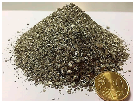
Figure 6. Highly pure Sn obtained by electrorefining.
