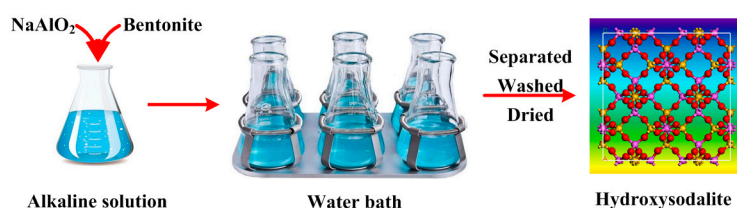
Figure 3. The flow diagram for the synthesis of hydroxysodalite.
