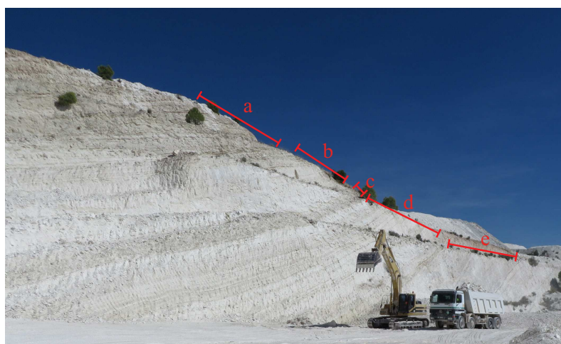
Figure 2. Active mine face section of the diatomite deposit where some of the ore samples were obtained: (a) limestone layer with small intercalations of diatomite; (b) diatomite layer with small intercalations of limestones; (c) limestone layer; (d) intercalation of diatomite, limestones, marls and clay horizons; (e) diatomite layer with small intercalations of limestones.
